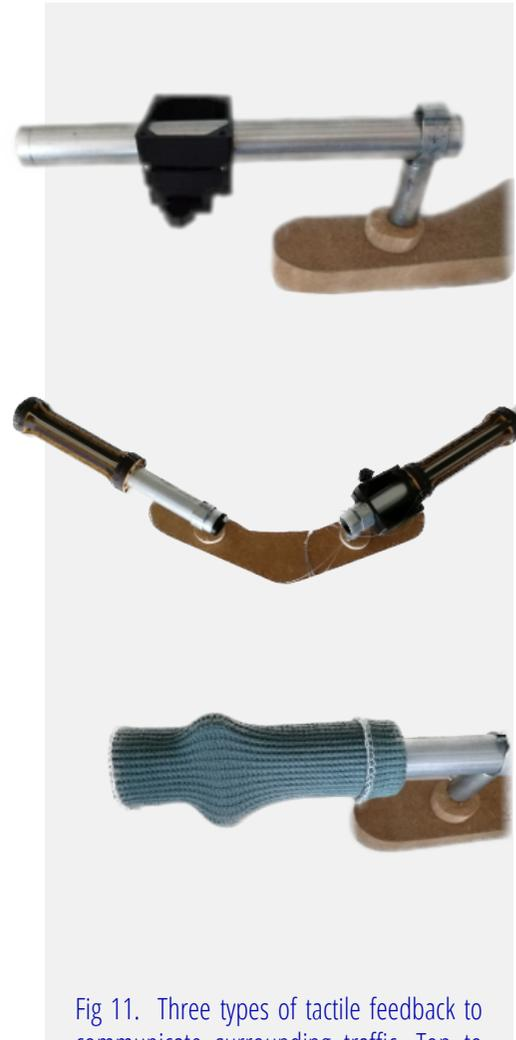
Fig 11. Three types of tactile feedback to communicate surrounding traffic. Top to bottom: force, motion and shape change.
