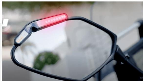
Fig 3. Motorcycle blind spot warning light on a mirror
