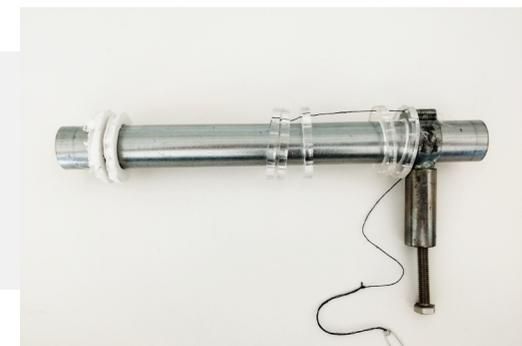
Fig 15. Motion feedback prototype. Motion achieved through sliding rings, actuated by strings.
