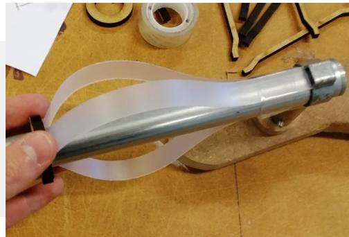
Fig 20. Shape change feedback prototype with akypop, a stronger flexible material.
