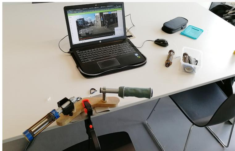
Fig 3. User test setup for validating tactile experiences.
