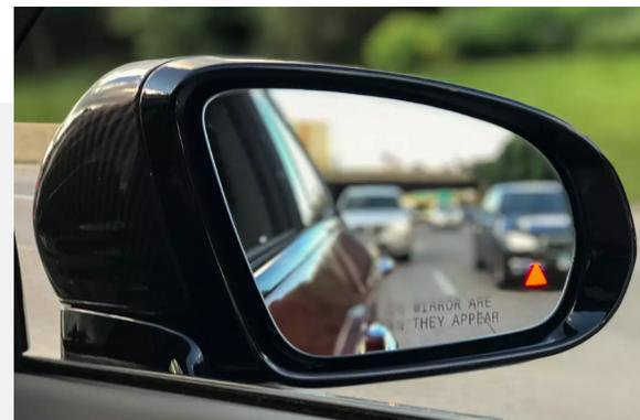
Fig 4. Blind spot warning light in car mirror.
