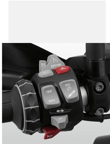
Fig 11. BMW handlebar controls offer extensive control options during riding, at the expense of (visual) attention to traffic.
